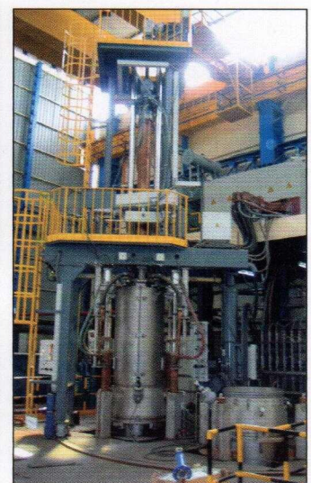
ESR Furnace with Inert atmosphere
