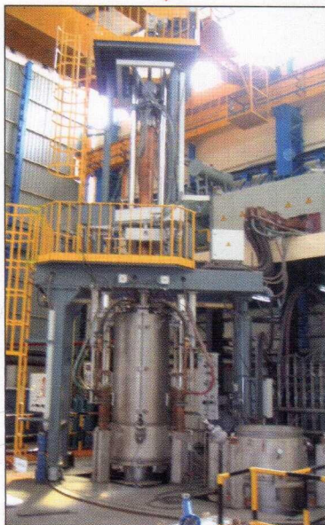
ESR Furnace with Inert atmosphere
