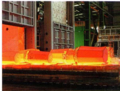
▲ Bogie Type Furnace
